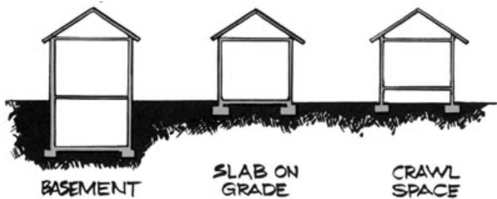
Radon reduction systems can be grouped by house foundation design. Find your type of foundation design above and read about which radon reduction systems may be best for your house.
